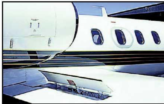
Spoilers reduce lift and increase drag during descent and landing.
